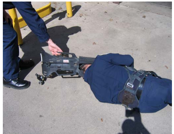
Crack At Lumbar Support Caused Seperation Failure
